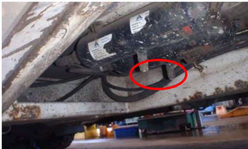
Damaged service brake reservoir fittings
